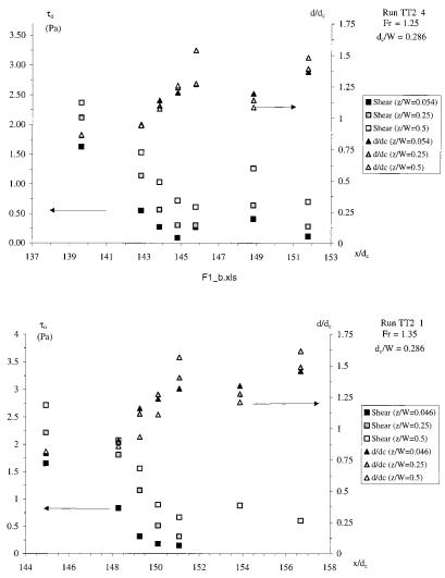
**Figure 1.** Bed shear stress along an undular hydraulic jump. (a) Flow conditions: Fr = 1.25,  $d_c/W = 0.286$ , W = 0.25 m (Run TT2\_4). (b) Flow conditions: Fr = 1.35,  $d_c/W = 0.286$ , W = 0.25 m (Run TT2\_1).
