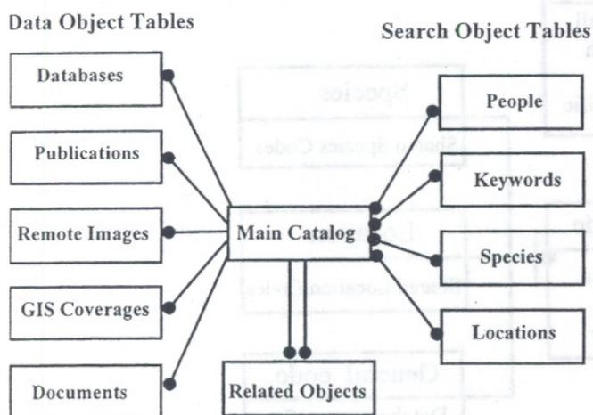
**Figure 1.**—A simplified structure including only the main entities and relationships of the FSDB Metadata Database (—• represents one-to-many relationships, •—• represents many-to-many relationships).
