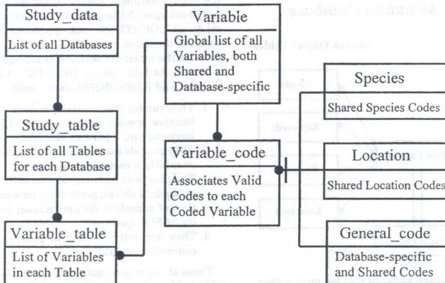
**Figure 3.**—The entities and relationships of the Study\_data Section of the FSDB Metadata Database. Relationships are all one-to-many, and the variable\_code table is sub-typed into three mutually exclusive tables.
