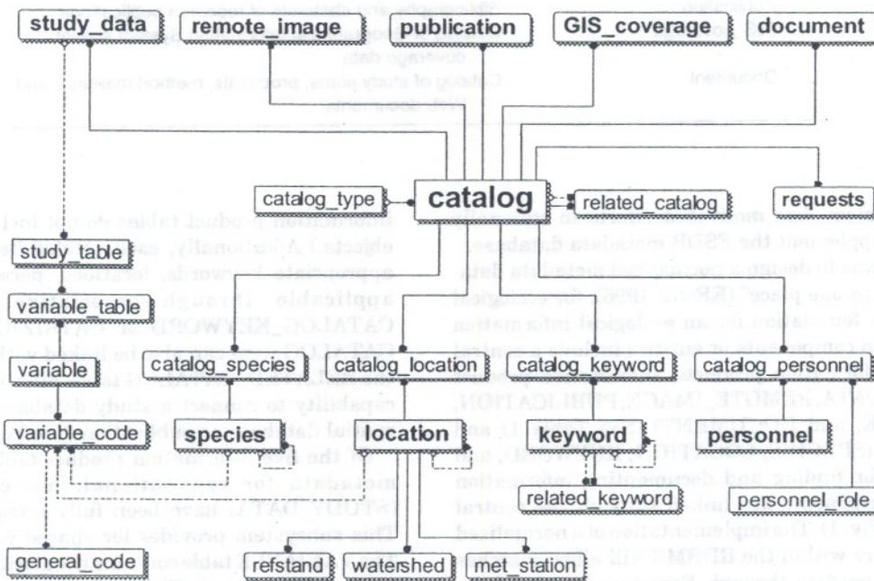
**Figure 2.**—Entity-Relationship diagram of the FSDB Metadata Database (—• represents one-to-many relationships; solid lines denote identifying relationships; dashed lines show non-identifying relationships, i.e., there is no identification dependency between two tables).
