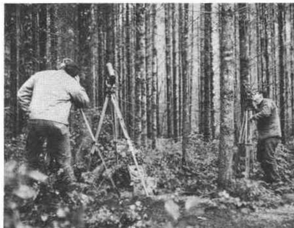
Figure 1. Instrument set-up for surveying spatial structures of trees. Two theodolites are in use; the instrument in the middle is a spotting laser.
