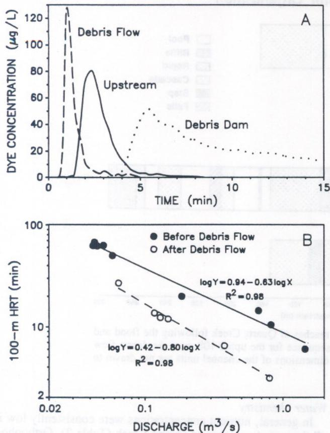
FIG. 4. Hydraulic features of Quartz Creek, determined from releases of fluorescein dye into the channel. (A) Dye concentration over time at 50 m downstream of the release point for the debris flow and upstream reaches, and within the debris accumulation; (B) 95% hydraulic residence time (HRT) for 100-m reaches in the debris flow reach, before and after the disturbance, at different discharges.
