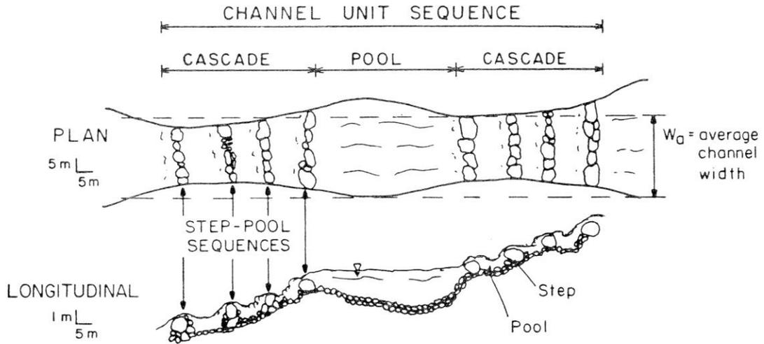
Fig. 2. Schematic diagram of channel morphology at the step-pool and channel unit scales.
