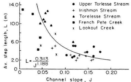
Fig. 3. Plot of step length versus channel slope; data points and curve for Torlesse and Irishman streams from Whittaker (1987).
