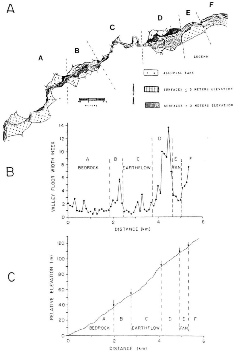
Fig. 7. Map of reaches and associated reach geometry along 5.5 km study area, Lookout Creek; 7A: planview of reaches and associated valley floor landforms; 7B: distribution of valley floor width index by reach type; 7C: longitudinal profile of the channel by reach type.
