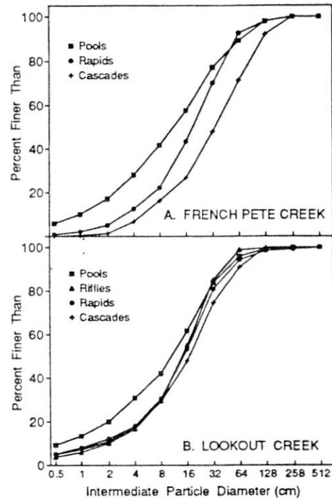
Fig. 5. Particle size distributions for French Pete and Lookout Creek channel units.
