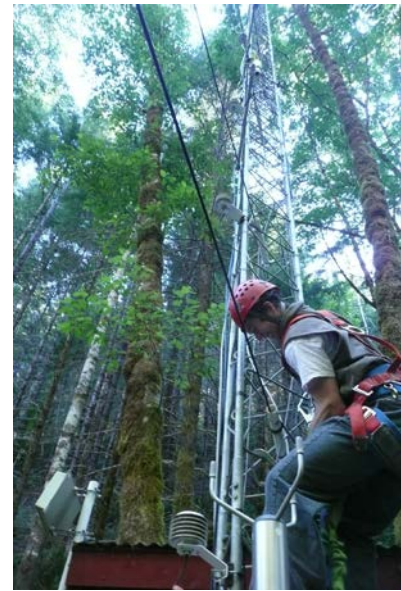
Figure II.B.12.1. A network of sensors on a 37m tower and an ecohydrological sensor network in WS1 provide high-spatial- and temporal-resolution environmental data that are conveyed by telemetry to the Andrews HQ and uploaded incrementally to the Andrews database. (M.S. student Scott Allen is shown in foreground)
